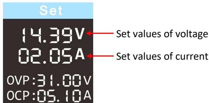
**Note:** The minimum of channel output current is 50mA
