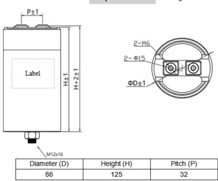
Dimensions in mm, unspecified dimensions tolerance ±1mm
