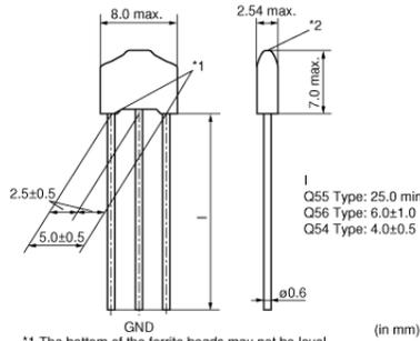
\*1 The bottom of the ferrite beads may not be level with each other.
