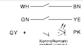
Contacts are shown in non-operated state (magnet is out of actuating distance Sar)
