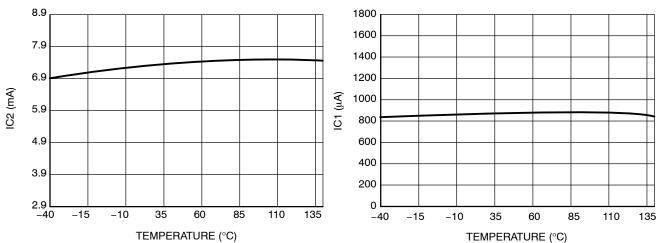
Figure 30. IC2 Startup Current vs. Temperature
