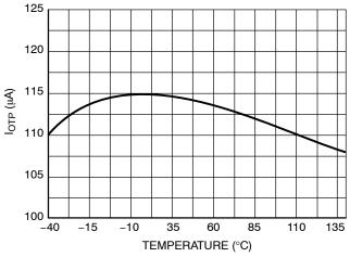
Figure 9. OTP Current vs. Temperature
