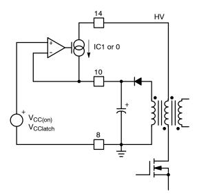
Figure 32. The Current Source Brings V<sub>CC</sub> Above 15 V (typical) and then Turns Off
