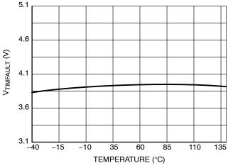
Figure 7. Fault Timer Level vs. Temperature
