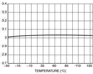
Figure 26. Latching Level vs. Temperature
