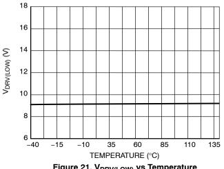
Figure 21. V<sub>DRV(LOW)</sub> vs Temperature
