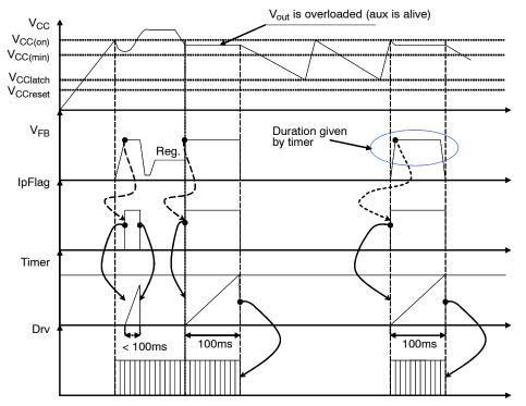
Figure 36. This Case is Similar to a Short-circuit where  $V_{\text{aux}}$  does NOT Collapse
