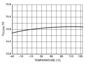
Figure 12. V<sub>CC(ON)</sub> Voltage vs Temperature
