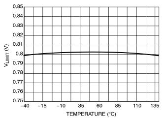
Figure 8. Current Sense Internal Setpoint vs. Temperature
