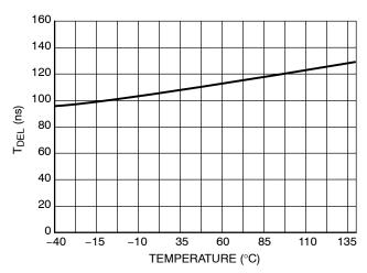
Figure 6. Propagation Delay vs. Temperature
