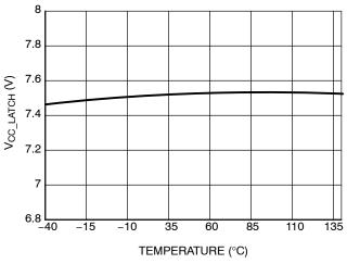
Figure 3.  $V_{CC}$  LATCH vs. Temperature
