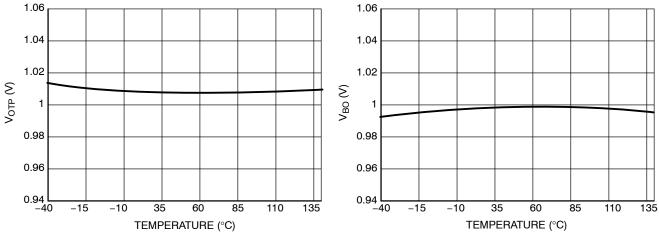
Figure 27. V<sub>OTP</sub> Voltage vs. Temperature
