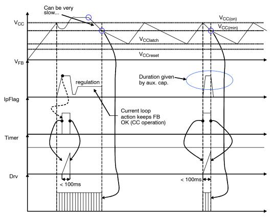
Figure 35. First Fault Mode Case
