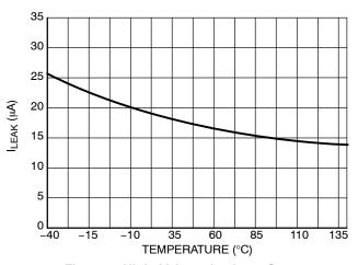
Figure 5. High-Voltage Leakage Curren vs. Temperature
