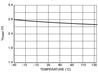
Figure 24. Ramp Level vs. Temperature
