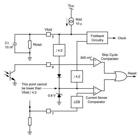
Figure 48. A Pulldown Resistor Adjusts the Foldback Level
