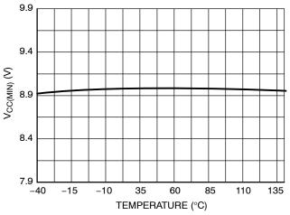
Figure 13.  $V_{CC(MIN)}$  Voltage vs Temperature
