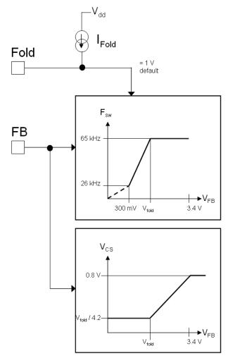
Figure 47. Operation in Light Load Conditions
