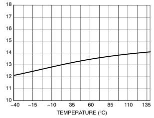
Figure 22. Drive Voltage  $V_{DRV(HIGH)}$  vs Temperature
