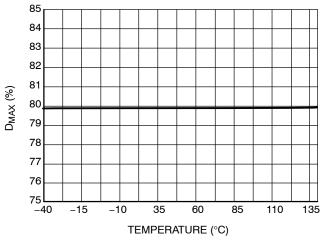
Figure 11. Maximum Duty-Cycle vs. Temperature
