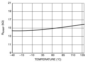
Figure 25. Ramp Resistor Value vs. Temperature
