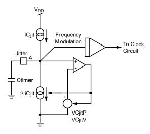
Figure 49. An Internal Ramp is Used to Introduce Frequency Jittering on the Oscillator Sawtooth
