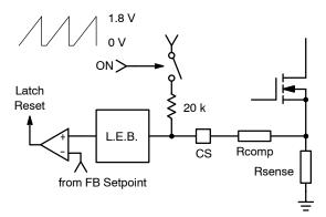
Figure 42. Inserting a Resistor
