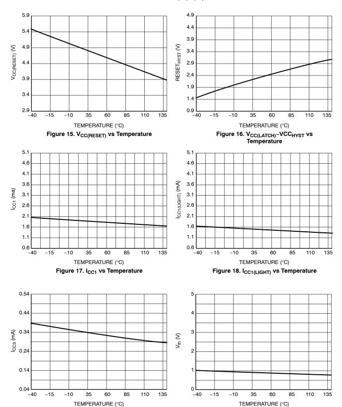
Figure 19. I<sub>CC3</sub> vs Temperature
