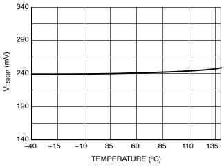
Figure 23. Skip Level vs. Temperature
