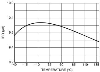
Figure 29. Brown-out Hysteresis Current vs. Temperature
