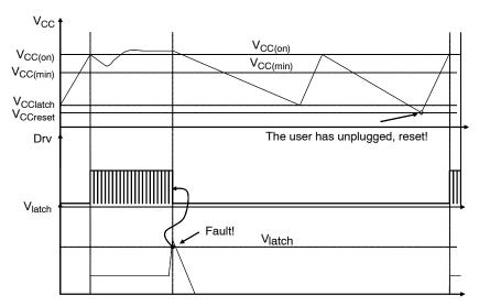
Figure 40. The Part is Reset when  $V_{CC}$  Reaches 5 V or when BO Senses the Bulk Capacitor Voltage is Back to Normal
