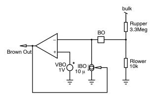
Figure 43. A Brown-out Circuit Protects the Power Supply against Low Input Voltages
