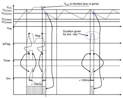
Figure 37. This Case is Similar to a Short-circuit where  $V_{\text{aux}}$  Does Collapse
