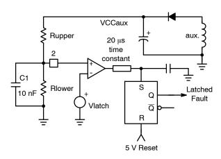
Figure 39. A Comparator Monitors Pin 2 and Latches-off the Part in Case the Threshold is Reached
