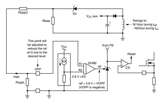
Figure 54. The Zener Diode can Introduce a Threshold which Disables OPP at Low Line for Maximum Power Capability
