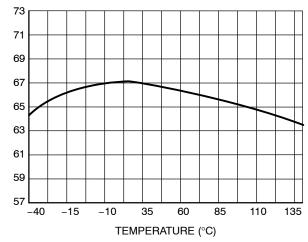
Figure 10. Oscillator Frequency vs. Temperature
