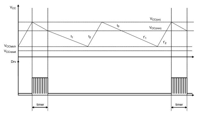
Figure 38. The Burst Period is Ensured by the  $V_{CC}$  Capacitor Charge / Discharge Cycle (here a 0.22  $\mu F$  capacitor on timer)
