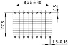
Hole arrangement View in mounting direction
