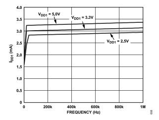
Figure 8. Typical  $I_{DD1}$  Current vs. Frequency, Duty = 50%,  $V_1$ + =  $V_{DD1}$
