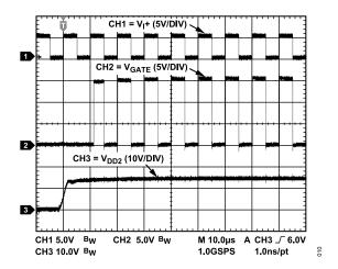
Figure 10. Typical V<sub>DD2</sub> Startup to Output Valid
