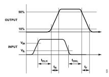
Figure 20. Propagation Delay Parameters
