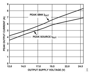
Figure 19. Typical Peak Output Current vs. Output Supply Voltage, 2  $\Omega$  Series Resistance ( $I_{OUT}$  is the Current Going into/out of the Device Gate)
