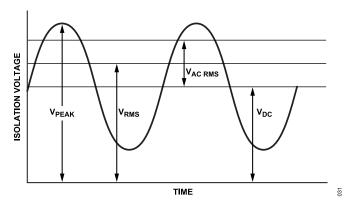
Figure 27. Critical Voltage Example
