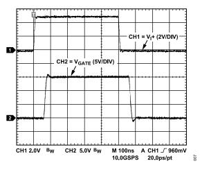
Figure 7. Typical Input to Output Waveform, 2 nF Load, 3.9  $\Omega$  Series Gate Resistor,  $V_{DD1}$  = 5 V,  $V_{DD2}$  = 15 V,  $V_{SS2}$  = 0 V
