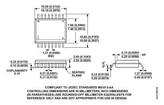
Figure 29. 16-Lead Standard Small Outline Package [SOIC\_W] Wide Body (RW-16)
