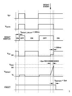
Figure 21. Desaturation Detection Timing Diagram
