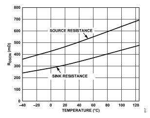
Figure 17. Typical Output Resistance ( $R_{DSON}$ ) vs. Temperature,  $V_{DD2}$  = 15 V, 1 A Test
