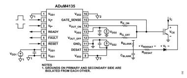
Figure 28. Typical Application Schematic
