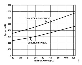
Figure 16. Typical Output Resistance ( $R_{DSON}$ ) vs. Temperature,  $V_{DD2}$  = 15 V, 250 mA Test
