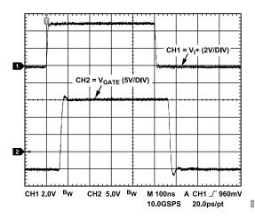
Figure 6. Typical Input to Output Waveform, 2 nF Load, 3.9  $\Omega$  Series Gate Resistor,  $V_{DD1}$  = +5 V,  $V_{DD2}$  = +15 V,  $V_{SS2}$  = -5 V
