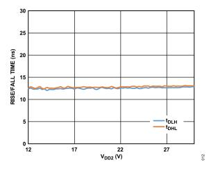
Figure 12. Typical Rise/Fall Time vs.  $V_{DD2},\,V_{DD1}$  = 5 V, 2 nF Load,  $R_{\rm G}$  = 3.9  $\Omega$
