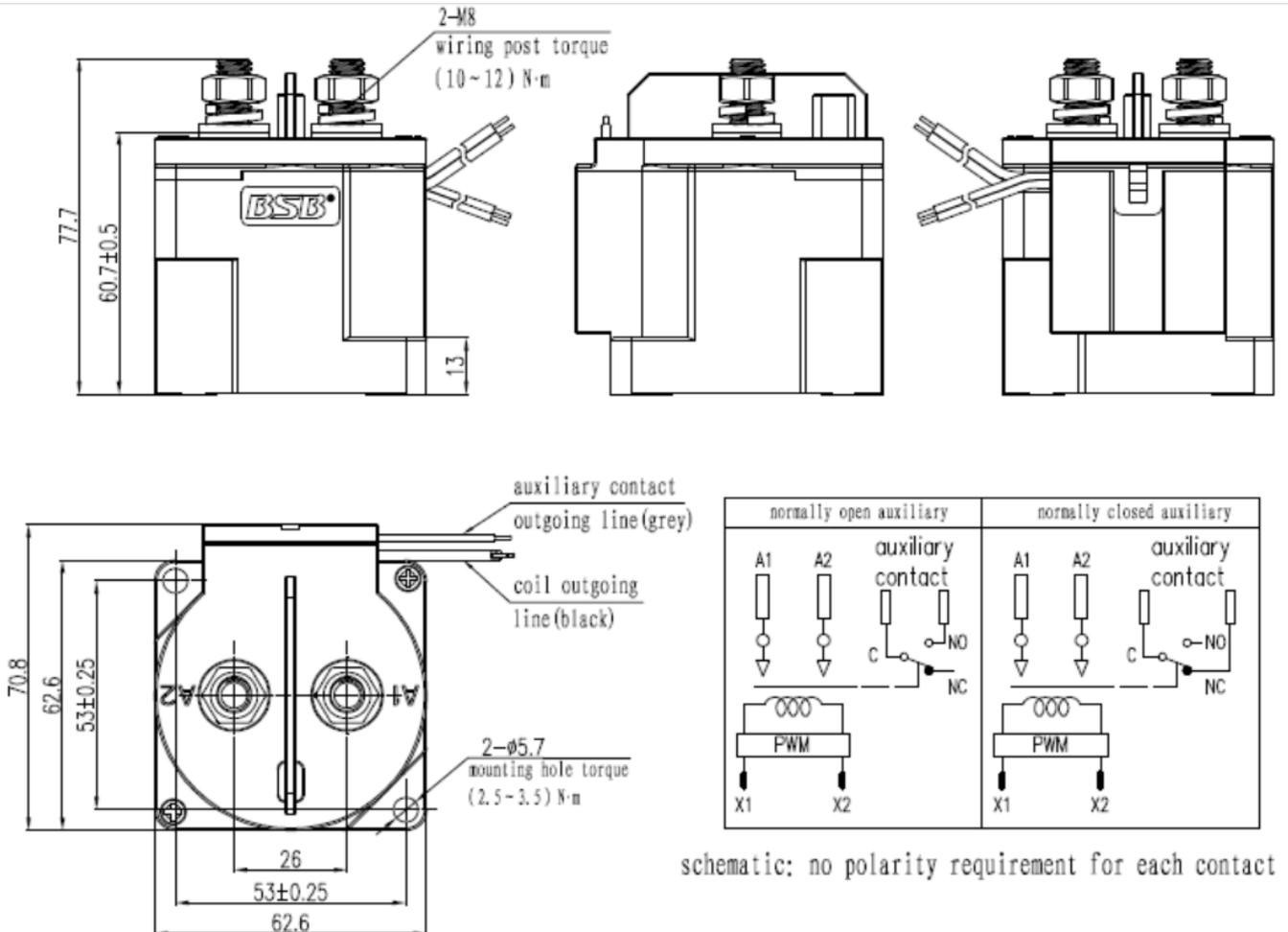
Note: Control coil wire length  $300\pm 20\text{mm}$
