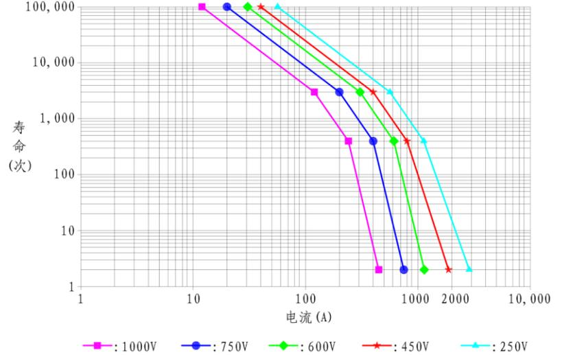
Note: Except for special note, the ambient temperature of electrical durability test is 23°C, and the on-break ratio is: 1s: 9s
