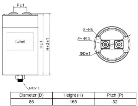
Dimensions in mm, unspecified dimensions tolerance ±1mm
