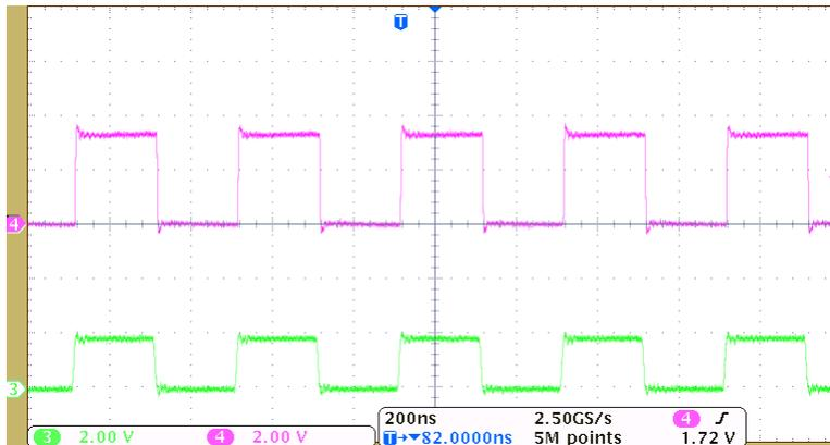
**Figure 7. Level-Translation of a 2.5-MHz Signal**
