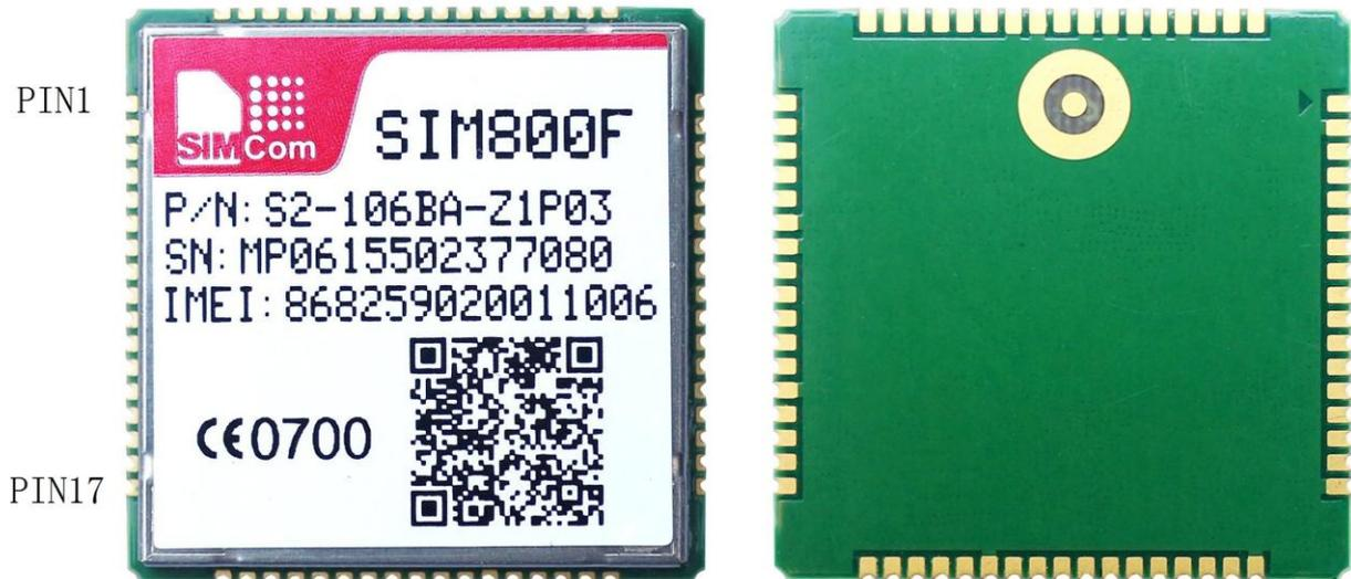
Figure 46: Top and bottom view of SIM800F
