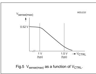
The maximum fixed frequency of the oscillator is set by an internal current source and capacitor. The maximum frequency is reduced once the control voltage enters the VCO control window. Then, the maximum frequency changes linearly with the control voltage until the minimum frequency is reached (see Figs 5 and 6).
