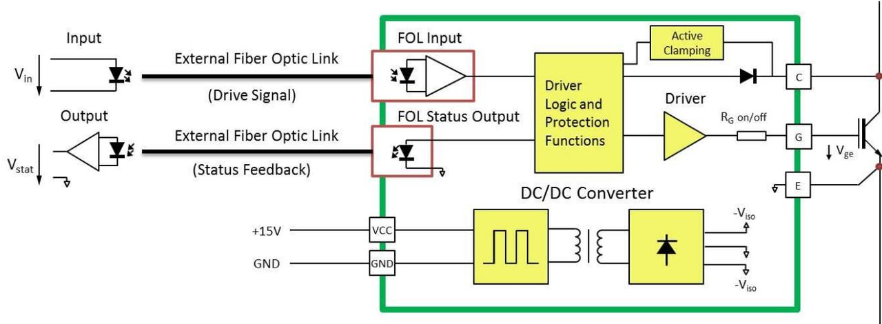
Figure 1: Basic schematic of the HPFM-HPM IGBT driver
