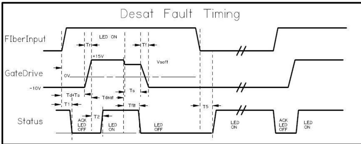
Figure 4: Signal fault timing diagram for Desat.
