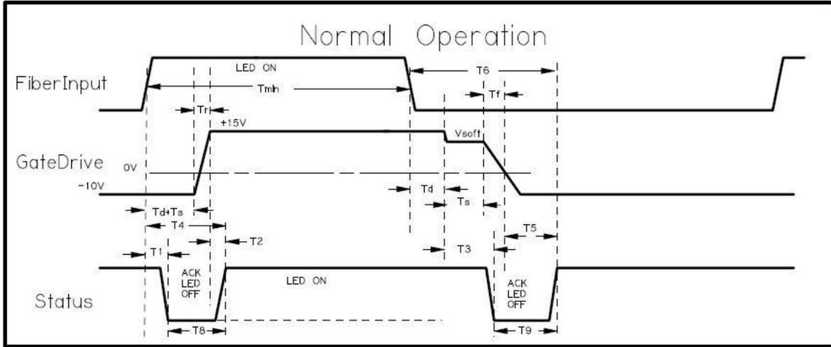
Figure 3: Signal input and output timing diagram
