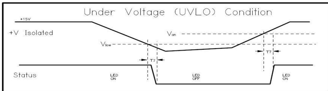
Figure 5: Signal fault timing diagram for UVLO.
